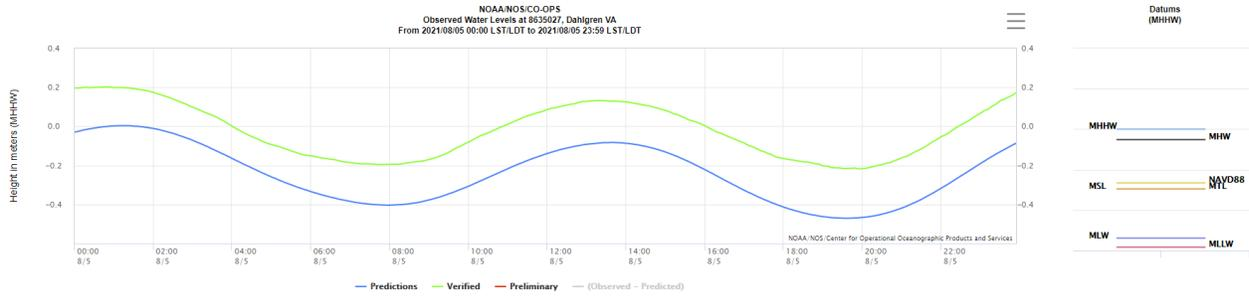
Figure 11 Tide Water level measurements at the NOAA tide gage at Dahlgren Station ID 8635027 was used to adjust the raw bathymetry of the hydrone data collection (i.e., tidal adjustment.) PI Allen developed a GIS script to automate this post-processing using coordinated timestamps from the tide gauge and hydrone GPS. <https://tidesandcurrents.noaa.gov/stationhome.html?id=8635027>.
