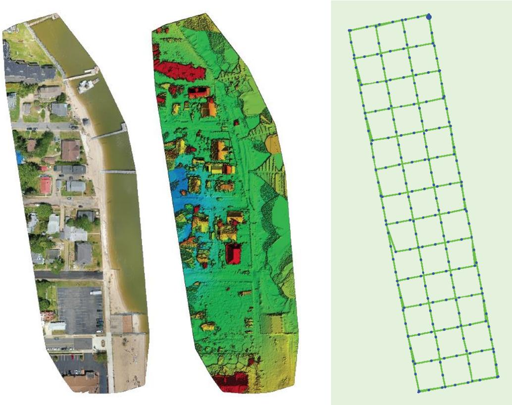
*Figure 3 Orthoimage mosaic (left), digital surface model (middle) and image tiles and tiepoints (right) developed by ODU GeoSEA.*
