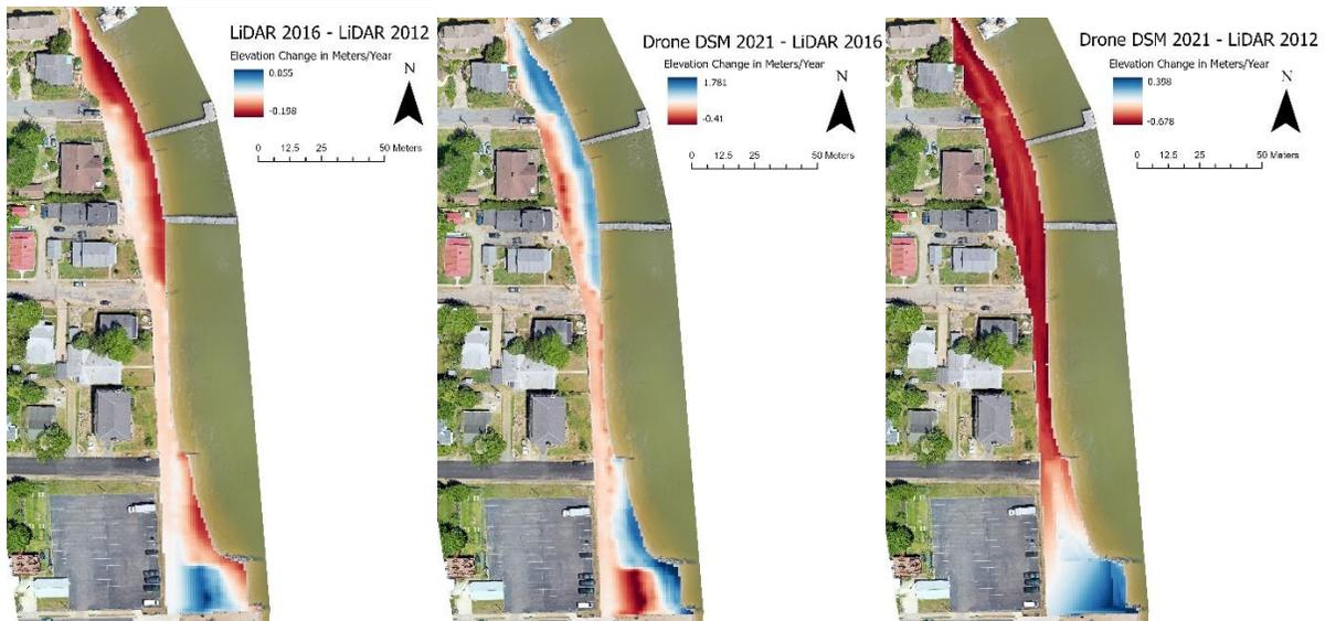
Figure 15 Time-sequential interval changes in beach elevations across the different LiDAR DEM and Drone DEM 2021 datasets depicts variability and cumulative erosion predominant change.
