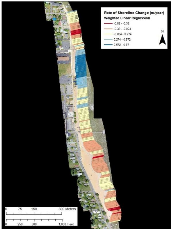
Figure 12 Map showing DSAS shoreline transects and derived shoreline change rates using the weighted linear regression technique. Hotspots of erosion are shown in oranges and reds while cool blues suggest low or even accretionary areas of change. Unsurprisingly, we quantified the locally known erosion in North Beach but also, surprisingly, indications of erosional trends around the breakwater beaches.
