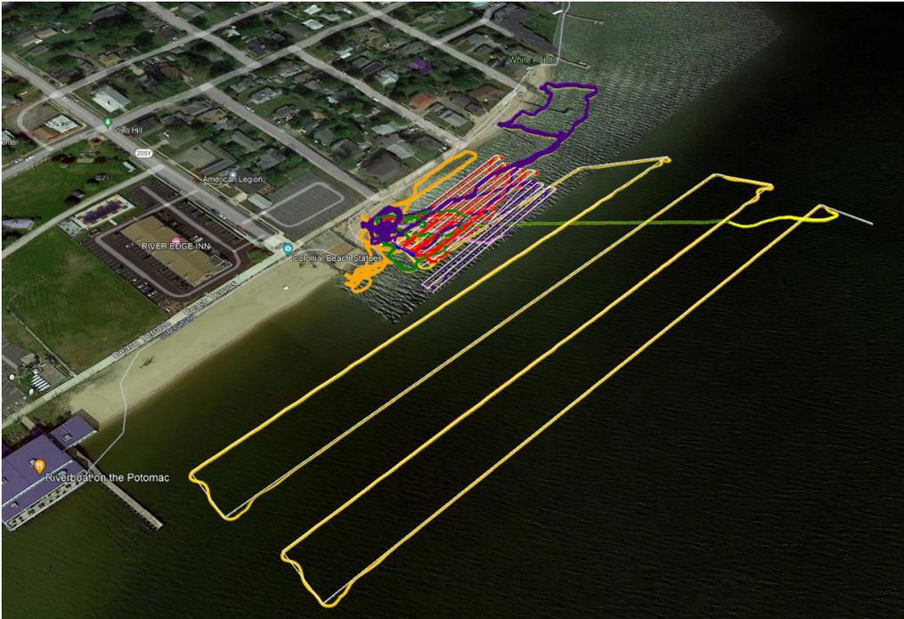
Figure 8 Missions planned and run by the Hydrone displayed in Gogole Earth Pro imagery. The various missions tested and verified the navigation, accuracy and alternative swath densities.
