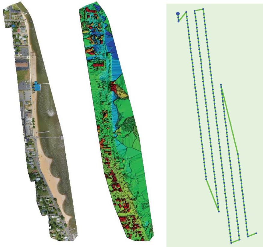
Figure 4 Study area site B to the south orthomosaic (left), surface model (middle), and flightline (right)
