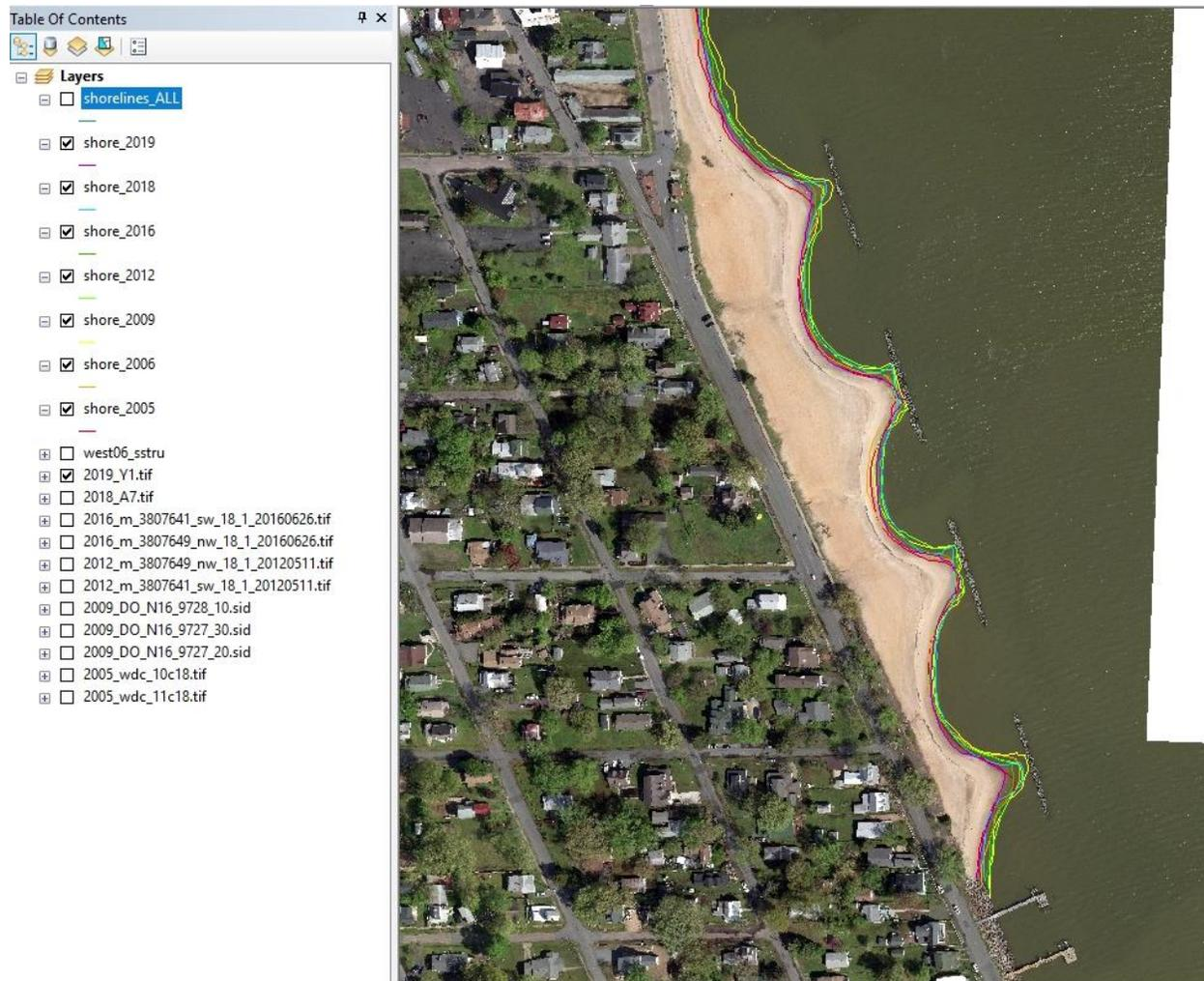
Figure 7 Site B shoreline digitization was also completed given the availability of the historic shorelines and new UAV orthoimagery. Since the UAV did not collect 3D mission data and drone data were cost prohibitive in time, the town and ODU consensus was to not derive volumetric analyses here. Further, a 3D UAV mission would have required direct overhead flights of beachgoers not allowed under FAA regulations.
