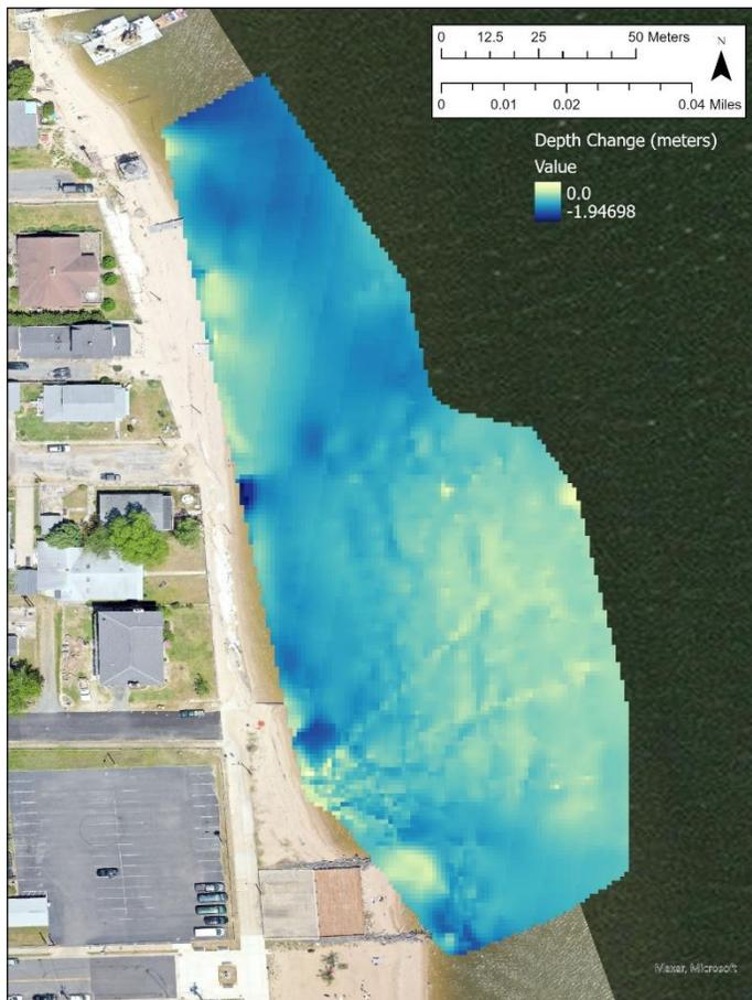
Figure 17 Map highlighting depth changes between 2012 Post-Irene topobathy LiDAR and 2021 Hydrone survey.
