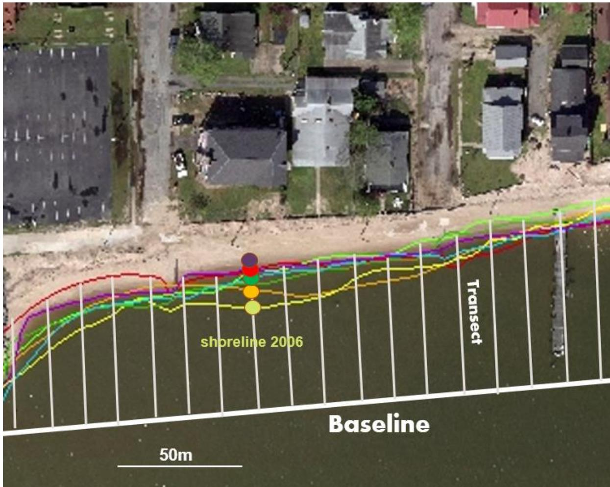
Figure 6 Methodology approach of DSAS consisted of digitizing an offshore baseline, casting perpendicular transects shoreward, and using these to intersect the historic and current shoreline positions. Each transect then has a distance and time component, allowing for calculation of shoreline change rates (SCRs.)
