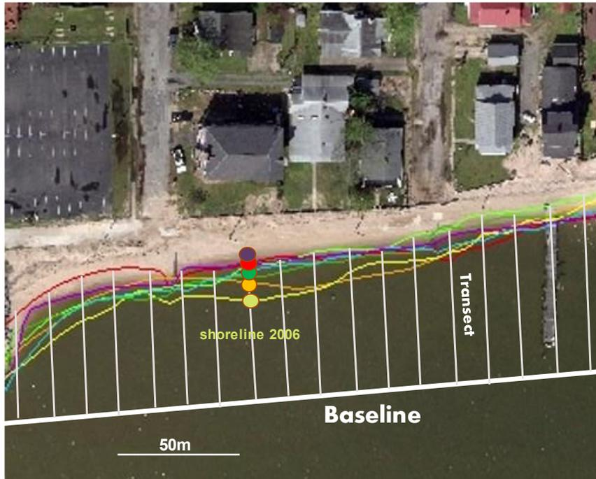
Figure 1 Shoreline Change Analysis features used by DSAS 5. This mockup shows the baseline and nominal shore-normal transects at North Beach with the intersected shorelines and transects allowing the measurement of changes and derivation of change rates (m/year)
