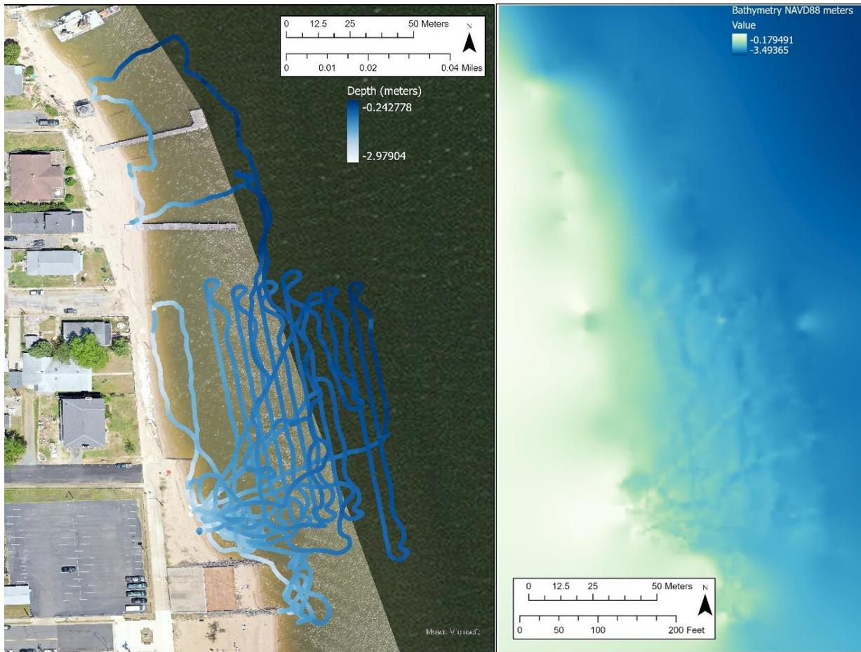
Figure 16 Final mission data for the Hydrone showing bathymetry depth points (left) after tidal correction prior to surface interpolation (right) displayed as a raster grid.
